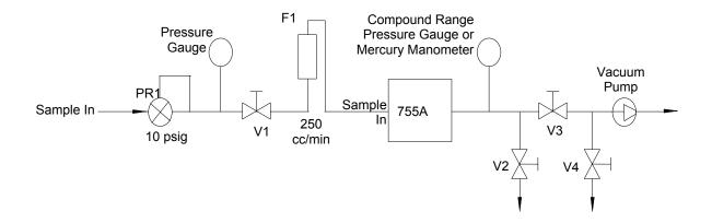
Figure 3-3. Calibration by Pressure Decrease Setup
